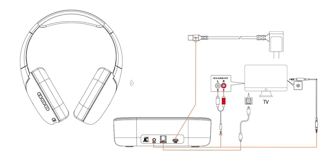
Use the Type-C adapter to connect the Base station for power supply
